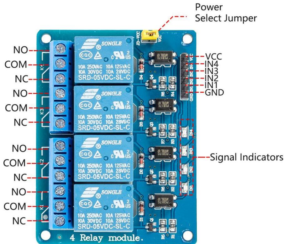
On the input side, where it receives the trigger signal, the connections typically include three or four pins, as outlined in the relay module circuit diagram:
