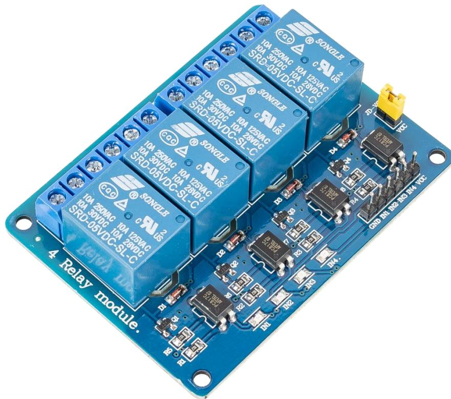
This is a LOW Level 5V 4-channel relay interface board, and each channel needs a 15-20mA driver current. It can be used to control various appliances and equipment with large current. It is equipped with high-current relays that work under AC250V 10A or DC30V 10A. It has a standard interface that can be controlled directly by micro-controller.
